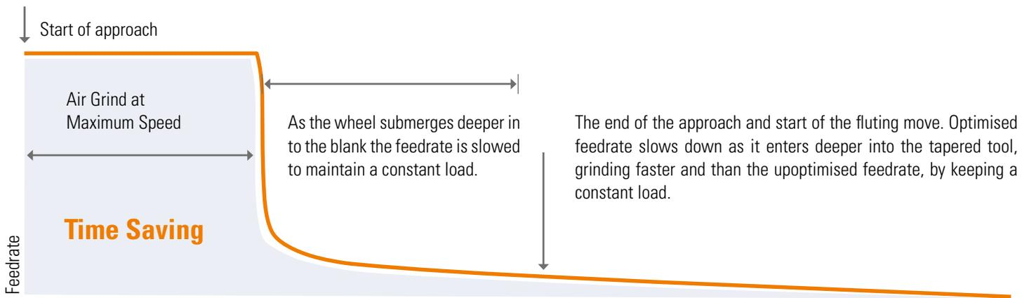
**The geometry of the tool is preserved as the axes positions remain untouched and only the feedrates are modified.**
